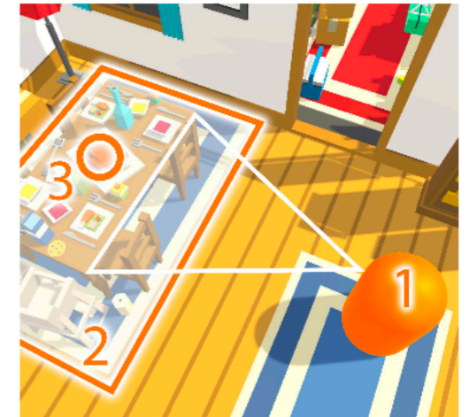
Figure 2: Gaze-supported player guidance in the game Lost and Found : if players (1) look at a gaze-sensitive area (2) where a game object is located (3), they get feedback via either visual, auditory, or haptic cues. The closer to the object, the stronger the feedback.
