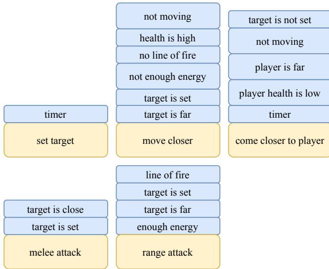
Fig. 4. Actions and corresponding decorators developed for Crew Member NPC's AI. Decorators are colored blue, actions are colored yellow.
